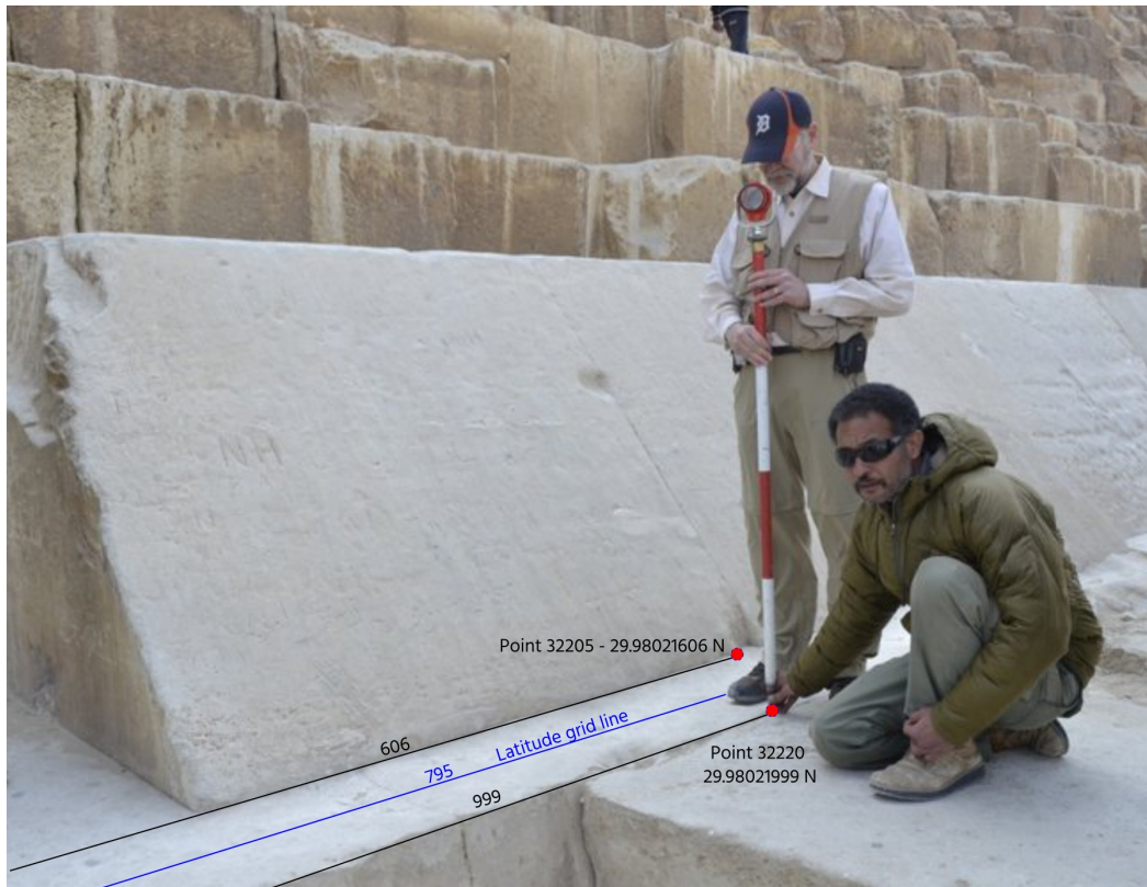
Diagram J-13 - The translated latitude grid line at the north face of the Great Pyramid.
